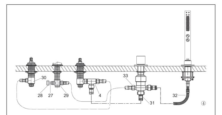
Put the fiber washer(27) into the plug(28), Tighten the plug to one of the ports of the center tee(29) for the spout.
